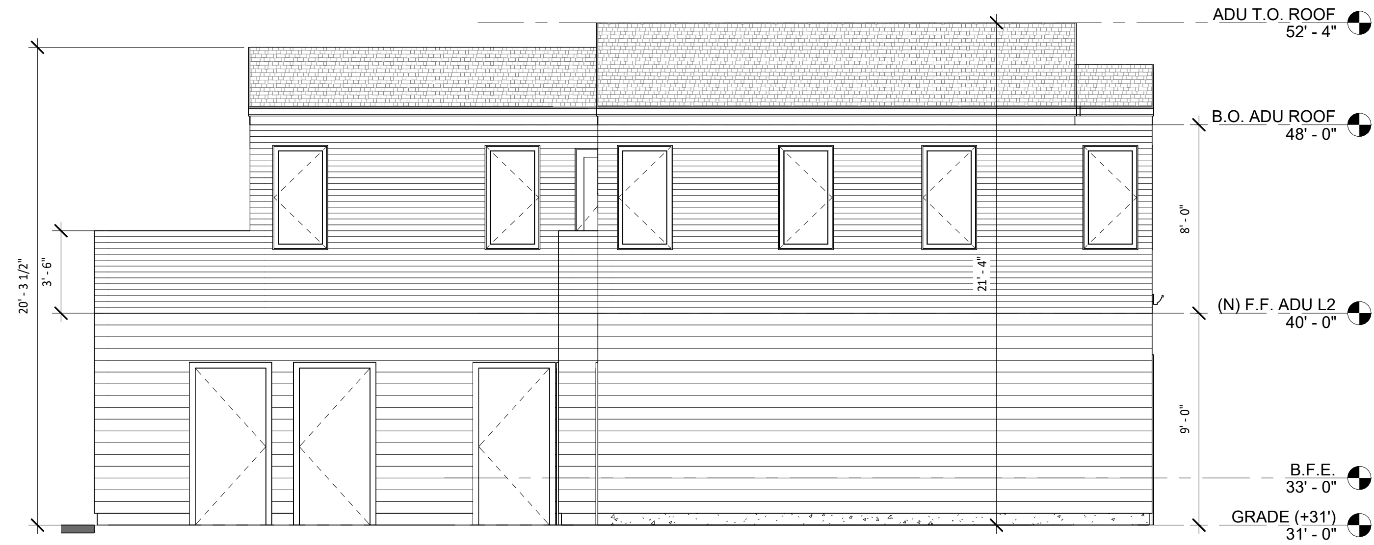
4 PROPOSED ADU ELEVATION - EAST SCALE : 1/4"=1'-0"
