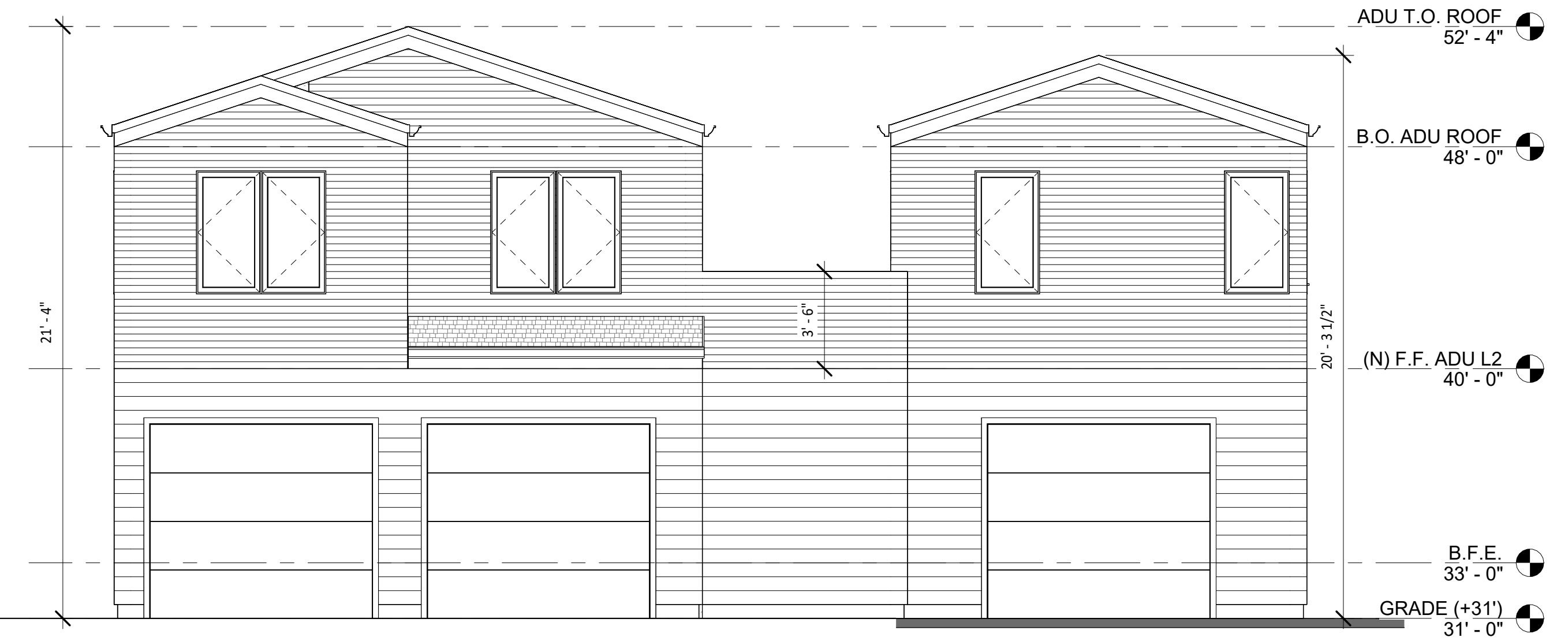
1 PROPOSED ADU ELEVATION - NORTH SCALE : 1/4"=1'-0"
