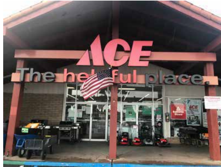
Suite 1056 - ACE - Channel Letters on exposed raceway (1) 6'-7" high x 22'-6" wide
