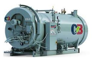
The boiler shall be a four-pass horizontal firetube updraft boiler with 5.0 square feet of heating surface per rated boiler horsepower. It shall be mounted on a heavy steel frame with an integrated forced draft burner and burner controls. The boilers shall be completely preassembled and fire tested at the factory. The unit shall be ready for immediate mounting on floor or simple foundation and ready for attachment of water, steam, fuel, electrical, vent and blow-down connections.
